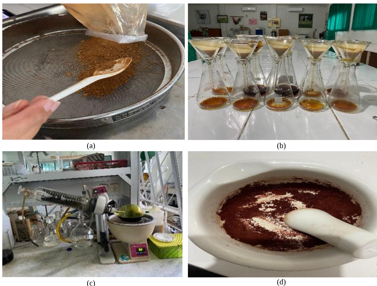
Figure 1. Preparation and extraction of bioactive compounds from cinnamon. a: Cinnamon powder filtering process, b: Filtration of the yield, c: Filtrate evaporation, d: Cinnamon extract grinding.
